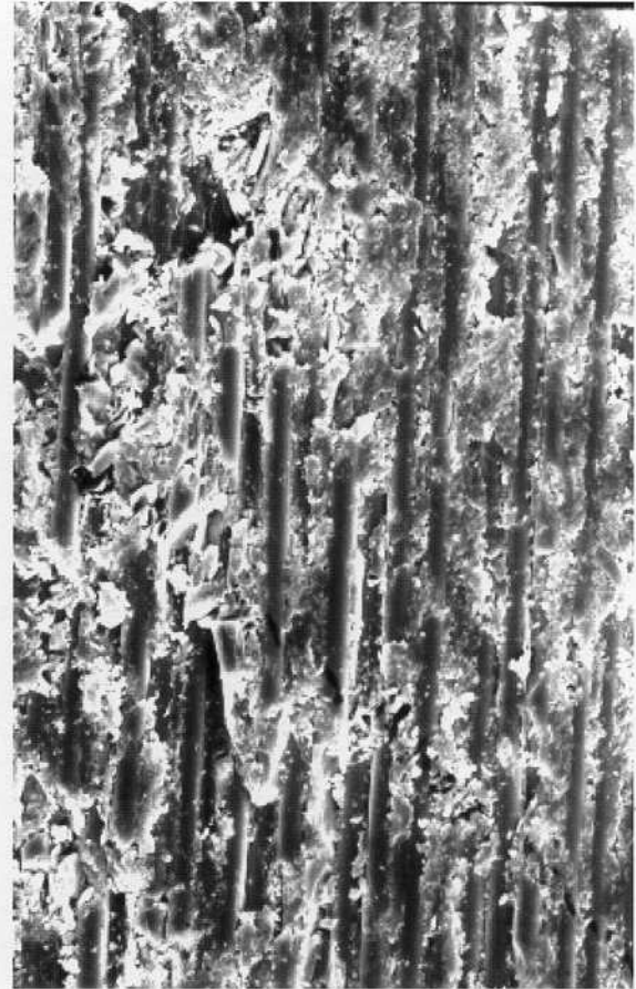
Figure 19. Slight Fiber Damage Caused by Thorough Sanding of Unidirectional Carbon-Epoxy Laminate
