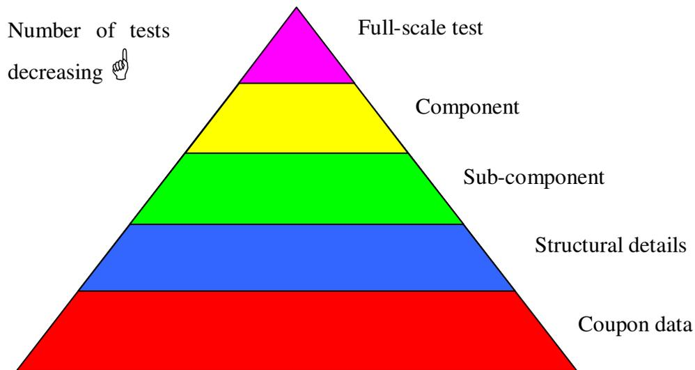
Figure 2. A schematic representation of the building block approach to certification of adhesive bonded structures.
