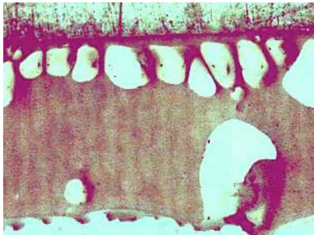
Figure 3: Excessive micro-voiding occurring adjacent to the end of one adherend, indicating the presence of micro-voids within the bond itself.
