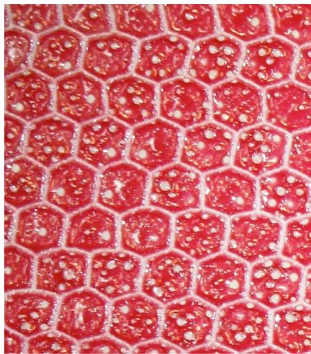
Figure 2: Micro-voids in sandwich structure. Note the occurrence of bubbles in the fillet areas of the bond, as well as in the centre of the cells.
